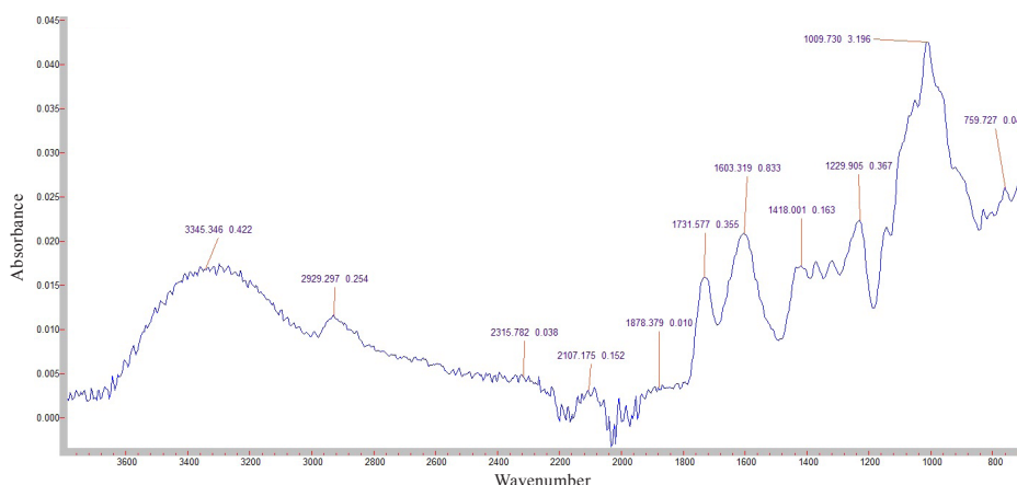
Figure 3 IR spectrum of pectin obtained by extracting with succinic acid in an ELF EMF
