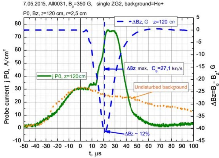
Figure 6. Sudden change in the background plasma and displacement of the external magnetic field; features of a slow magnetosonic wave.  $B_0=350$  G, laser ZG2, helium background. Coordinates of the P0 and Bz probes:  $r=2.5$  cm,  $z=120$  cm
