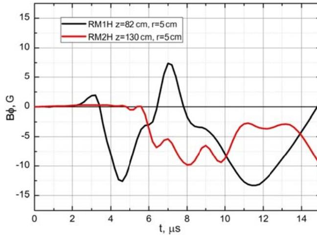
Figure 7. Disturbance of the  $B_0$  field at different distances  $z$  from the target.  $B_0=175$  G, double laser pulse LUI+ZG2, 3.3  $\mu$ s time delay between pulses, helium background. Coordinates of the probes: RM1H —  $r=5$  cm,  $z=82$  cm; RM2H —  $r=5$  cm,  $z=130$  cm
