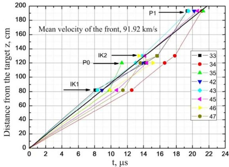
Figure 3. R–t diagram for the LP cloud in vacuum with magnetic field.  $B_0=100$  G, laser ZG2, vacuum
