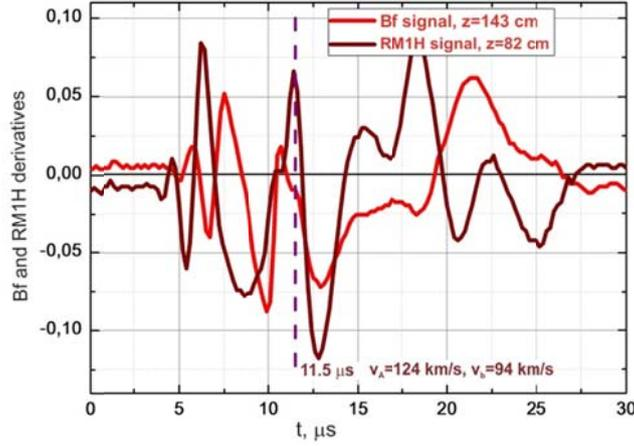
Figure 12. Derivatives of variations in the  $B_\phi$  magnetic field at different distances from the target.  $B_0=175$  G, laser LUI, hydrogen background,  $V_b=30$  km/s
