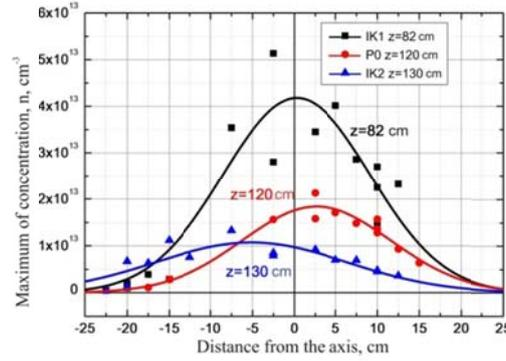
Figure 2. Radial distribution of plasma concentration at different distances  $z$  from the target.  $B_0=350$  G, the double laser pulse ZG2+LUI, 10  $\mu$ s time delay between pulses, vacuum, maximum plasma concentration  $\sim 30$   $\mu$ s after the pulse
