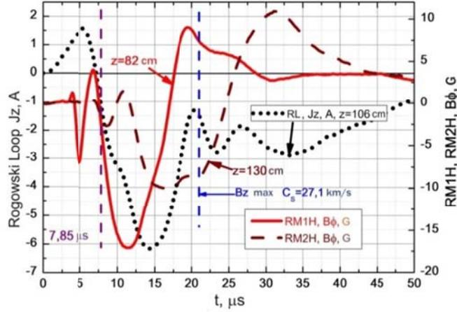
Figure 5. Disturbances of the  $B_0$  magnetic field and  $J_z$  current, AW features.  $B_0=175$  G, laser ZG2, helium background. Coordinates of the detectors: RM1H —  $r=5$  cm,  $z=82$  cm; RL —  $r=0$  cm,  $z=106$  cm; RM2H —  $r=5$  cm,  $z=130$  cm
