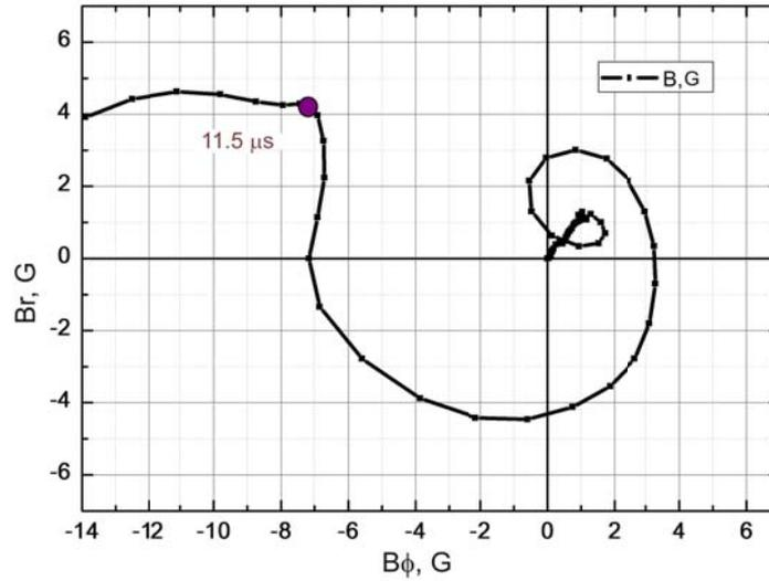
Figure 9. The hodograph of the transverse magnetic field component. The right-hand whistler polarization transforms into the left-hand AW polarization.  $B_0=175$  G, laser LUI, hydrogen background
