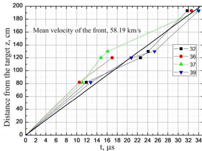
Figure 4. R–t diagram for the LP cloud in the background (helium).  $B_0=100$  G, laser ZG2
