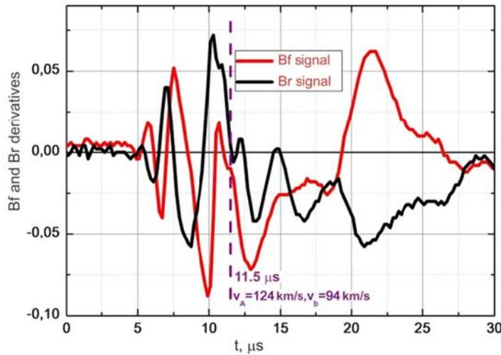
Figure 10. Derivatives of variations in the  $B_\phi$ ,  $B_r$  magnetic fields, the whistler predictor.  $B_0=175$  G, laser LUI, hydrogen background,  $V_b=30$  km/s
