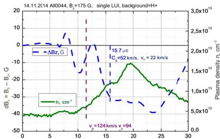
Figure 11. BP concentration change and displacement of the  $B_z$  field.  $B_0=175$  G, laser LUI, hydrogen background,  $V_b=30$  km/s
