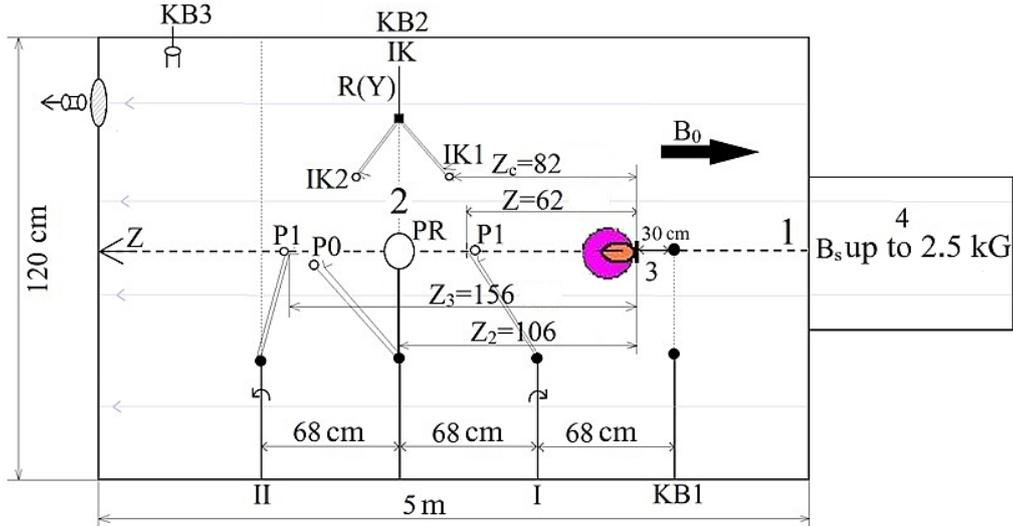
Figure 1. Diagram of the experimental stand KI-1: 1 is a symmetry axis of the chamber; 2 is a central section of the chamber; 3 is a laser target; 4 is  $\theta$ -pinch. The diagram shows two positions of the P1 probe at different stages of the experiment
