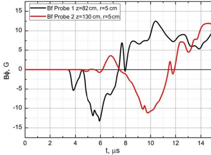
*Figure 8.* Disturbances of the  $B_\phi$  field according to the computer model data. There is a similarity with experimental data presented in Figure 7 in signal amplitude and time of its arrival at the probes
