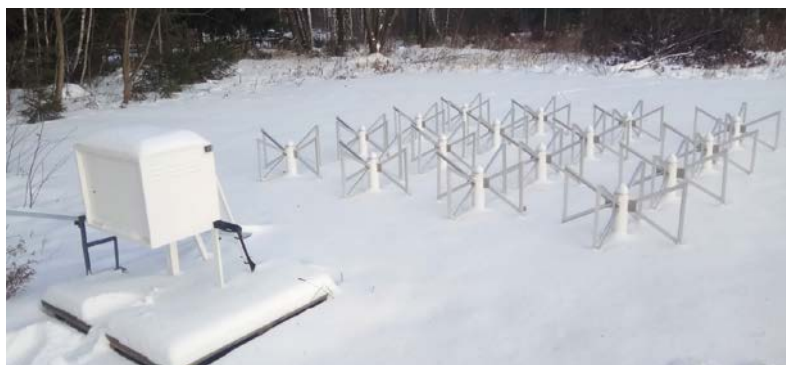
Figure 5. Prototype of the 4\times 4 antenna module
