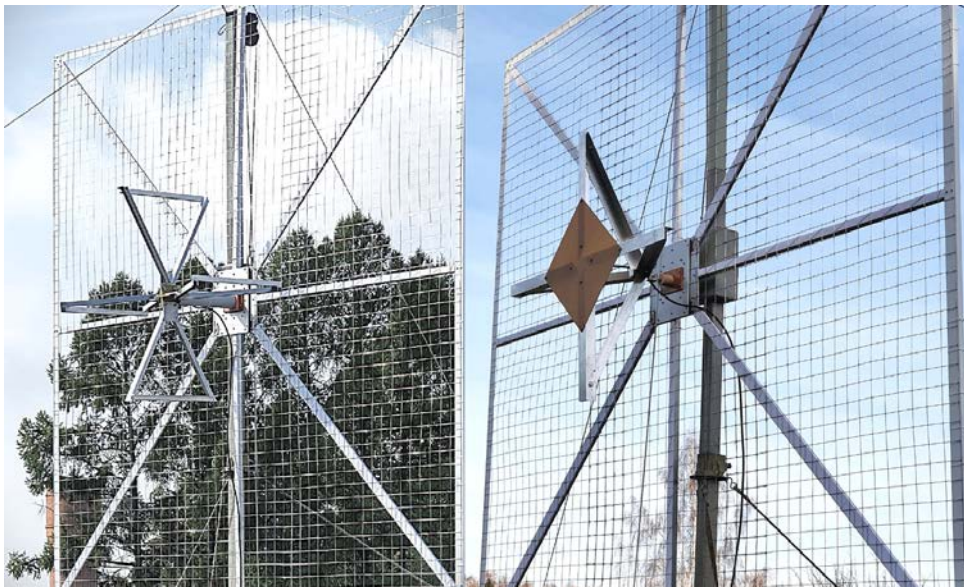
Figure 2. Antenna elements “bowtie” (left) and “delta” (right) on a test bench
