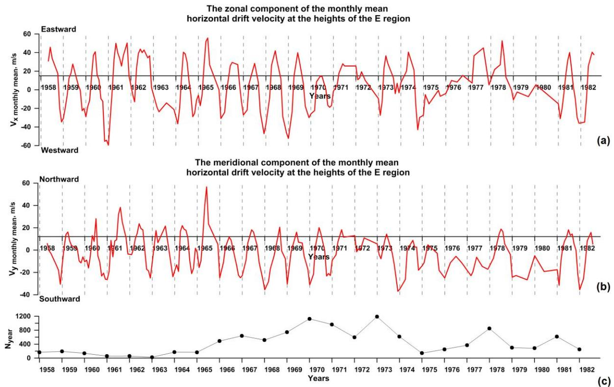
Figure 3. Zonal (a) and meridional (b) components (smoothed over three months) of the monthly mean horizontal drift velocity in the E-region; the number of annual average measurements in the E-region (c)
