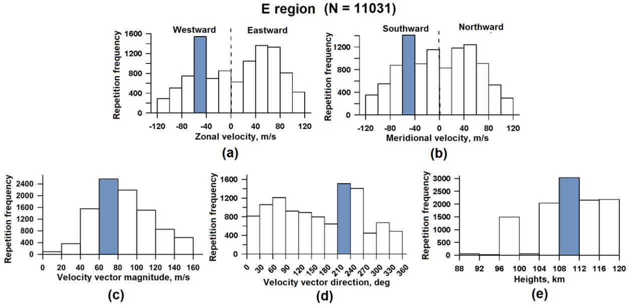
Figure 5. Frequency histograms of the zonal  $V_x$  (a) and meridional  $V_y$  (b) components, the modulus (c) and direction (d) of the ionization irregularity drift velocity vector, as well as the signal reflection altitude (e) for the E-region
