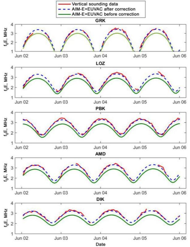
Figure 5. Diurnal variation of regular E-layer critical frequencies ( $f_oE$ ) on June 2–5, 2015: red lines are observations at GRK, LOZ, PBK, AMD, and DIK; solid green and blue dashed lines indicate results of AIM-E calculations from the EUVAC photon flux before and after correction respectively
