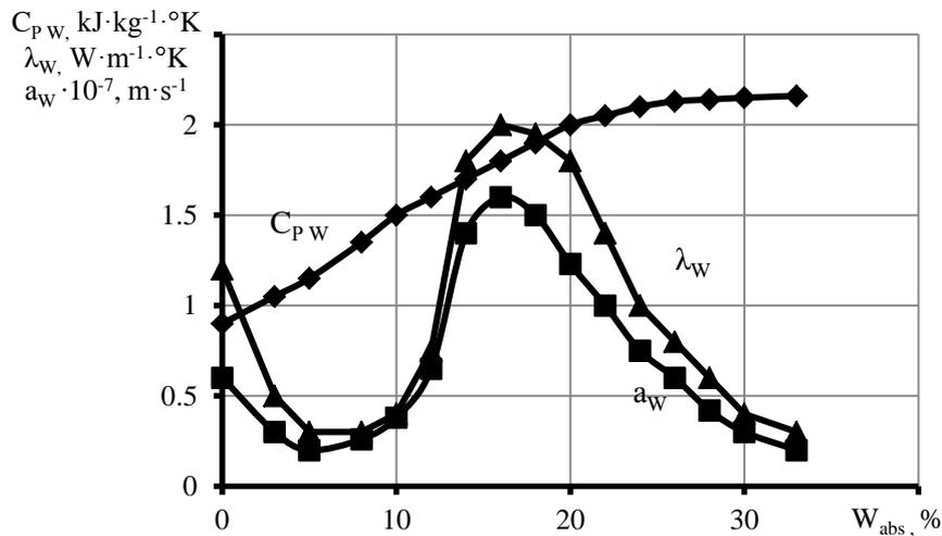
**Fig. 1.** Relation between thermophysical properties and moisture content of material.
