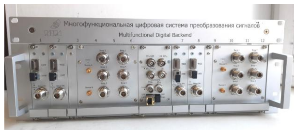
Figure 2. Four-channel MDBE system for radio telescopes RT-32
